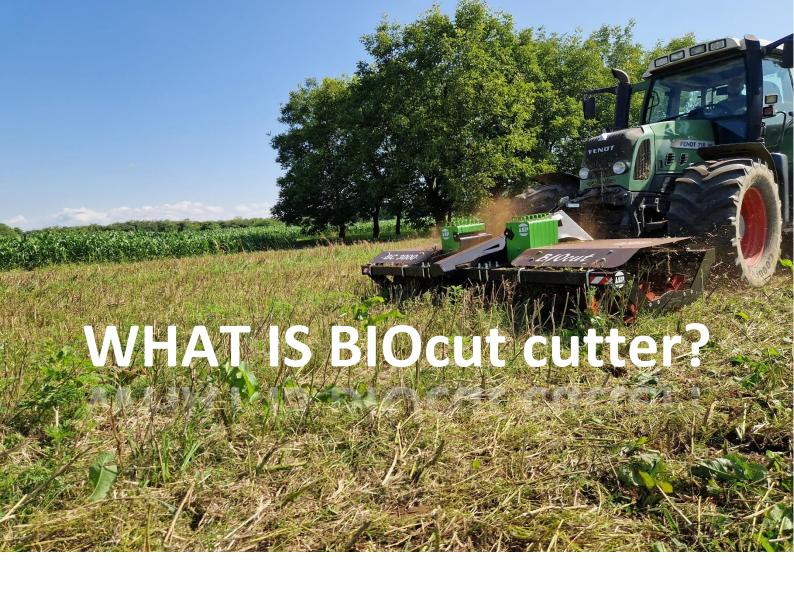
BIOcut cutter is roller equipped with knives whose main purpose is to allow the user to mow the crops at the end of the cycle. Rolling and crimping actions will transform crops into a thick weed suppressing mulch.
