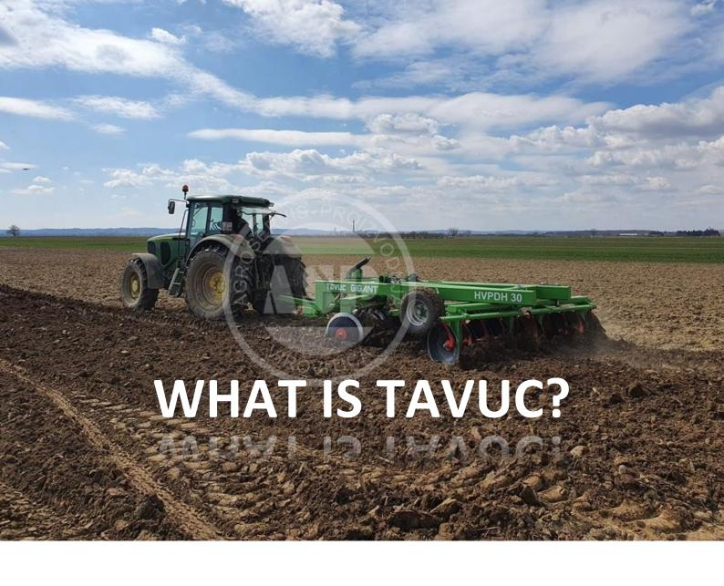
**TAVUC** is trailed machine inteded for pre - sowing operations on soil, to chop residues, stubble management and leveling smaller microdepressions.
