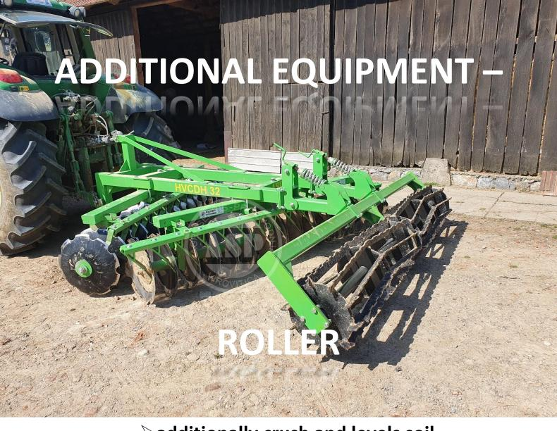
➤ additionally crush and levels soil➤ adjustable working depth
